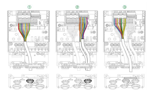
NOTE: Cabling plate shown is for frame size 2. Other cabling plates look slightly differs from this one. NOTE: For Floor standing products route the control wires into the integrated control cable conduit.
