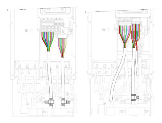
Example: cable path for frame size 5Y for 500-690 V mains voltage
