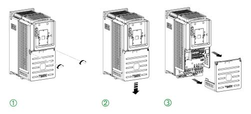
Apply the following instructions to access the terminals on frame sizes 1 to 3 IP20 drives
