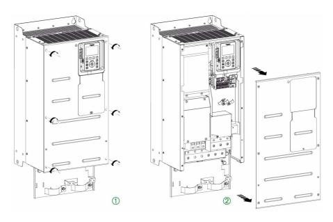
Apply the following instructions to access the terminals on frame sizes 3Y and 5Y drives
