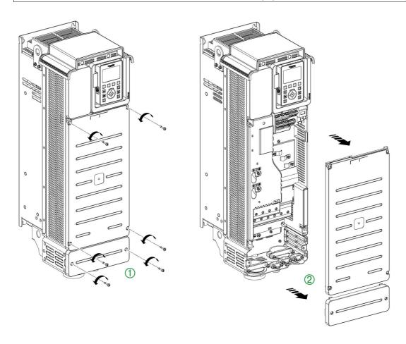
Apply the following instructions to access the terminals on frame sizes 4 and 5 drives
