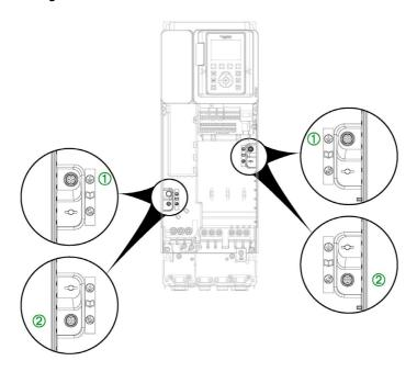
Setting For Frame Size 3S, Frame Size 3Y and Frame Size 4 Products, 200...240  $\rm V$
