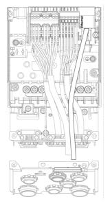
plates Ir NOTE: Cabling plate shown is for frame size 2. Other cabling plates look slightly differs from this one. NOTE: For Floor standing products route the control wires into the integrated control cable conduit.
