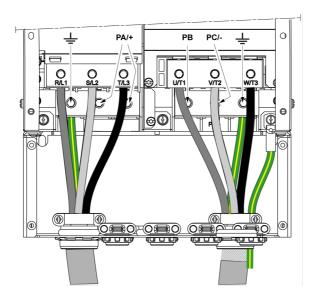
**NOTE:** PA/+ and PC/- terminals are used only to measure the DC Bus voltage and are not intended to be wired for an external use.
