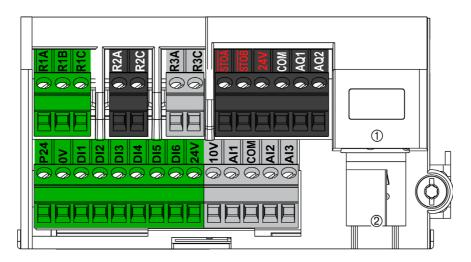
1 Ethernet Modbus TCP, 2 Serial Modbus
