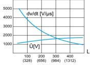
L Length of motor cables in meters (feet)
