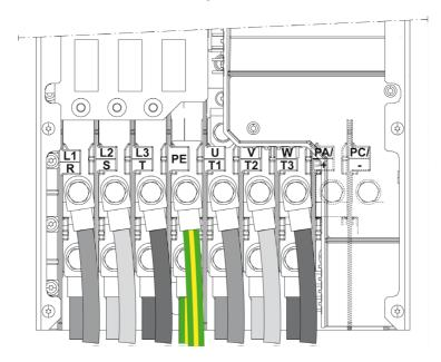
NOTE: PA/+ and PC/- terminals are used only to measure the DC Bus voltage and are not intended to be wired for an external use.
