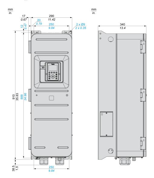
IP55 / UL Type 1 Drives With Load Switch - Front and Side View
