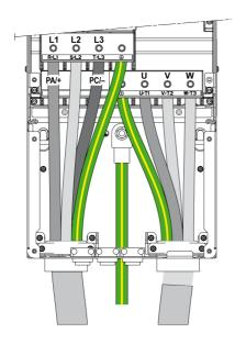
**NOTE:** PA/+ and PC/- terminals are used only to measure the DC Bus voltage and are not intended to be wired for an external use.
