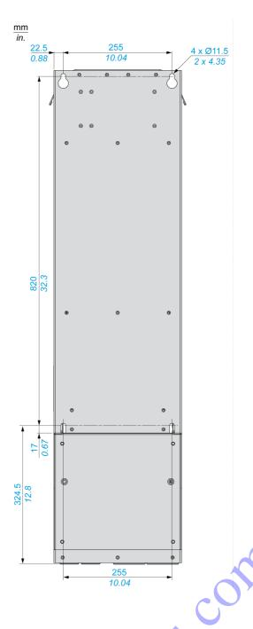
NOTE: Lower Conduit Box part sold separately. This part enables wall mounting of the product. It provides IP21 protection degree on the bottom side and UL type 1 protection degree.
