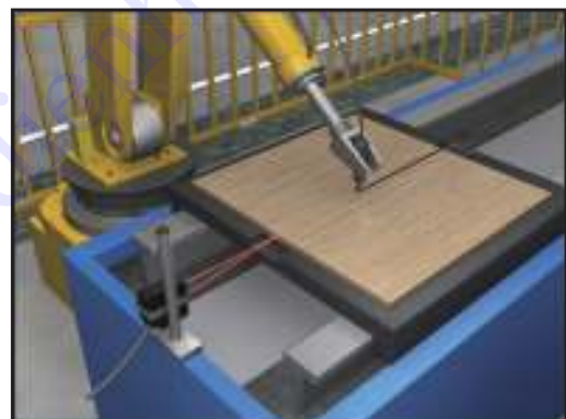
Workpiece detection for woodworking machines
