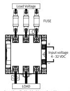
\*\* Fuse is not installed inside this product. We suggest you to use fasr-acting fuse outside separately like the picture.
