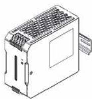
(A) Standard (Vertical) mounting
