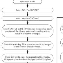
Press the Set-key to select the decimal point position of the prescale value. (Select the decimal point of the prescale value in the lower 5th digit) Prescale value setting with front SV 2—stage setting switch (Set the SV 2nd stage setting switch to '0.09425')
