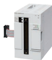
Differential driver output type FX5-20PG-D
