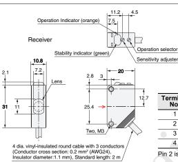
Terminal No. Specifications +V 2 3 0V 4 Output Pin 2 is not used.
