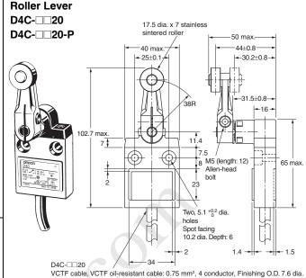
SJT(O) cable; 0.83 mm², 4 conductor, Finishing O.D. 8.6 dia. D4C-\( \subseteq 20-P\) (Weather-resistant Models) VCTF oil-resistant cable\*: 0.75 mm², 4 conductor, Finishing O.D. 7.6 dia. VCTF oil-resistant cable only
