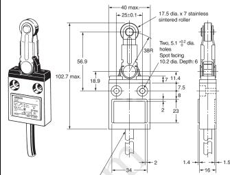
VCTF cable, VCTF oil-resistant cable: 0.75 mm², 4 conductor, Finishing O.D. 7.6 dia. SJT(O) cable: 0.83 mm<sup>2</sup>, 4 conductor, Finishing O.D. 8.6 dia.
