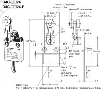
VCTF cable, VCTF oil-resistant cable: 0.75 mm², 4 conductor, Finishing O.D. 7.6 dia. SJT(O) cable: 0.83 mm2, 4 conductor, Finishing O.D. 8.6 dia.
