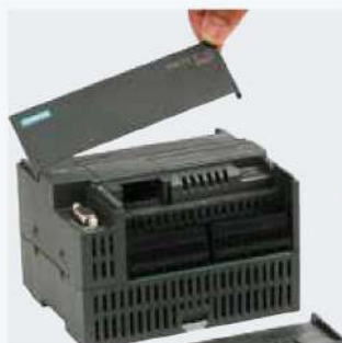
Remove the cover board of terminal
